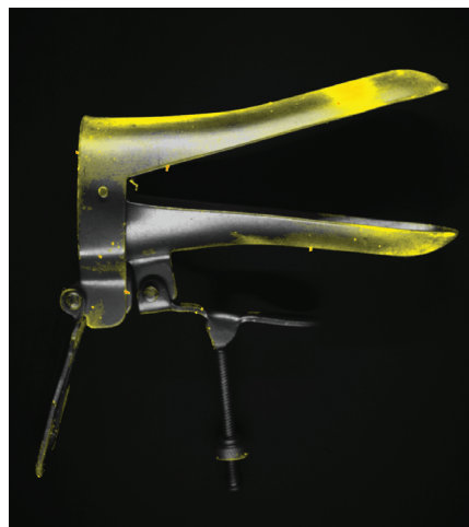
The most consistent problem highlighted by the ProReveal system is unidentified manufacturing debris and protein on ready to use sterile instruments.
